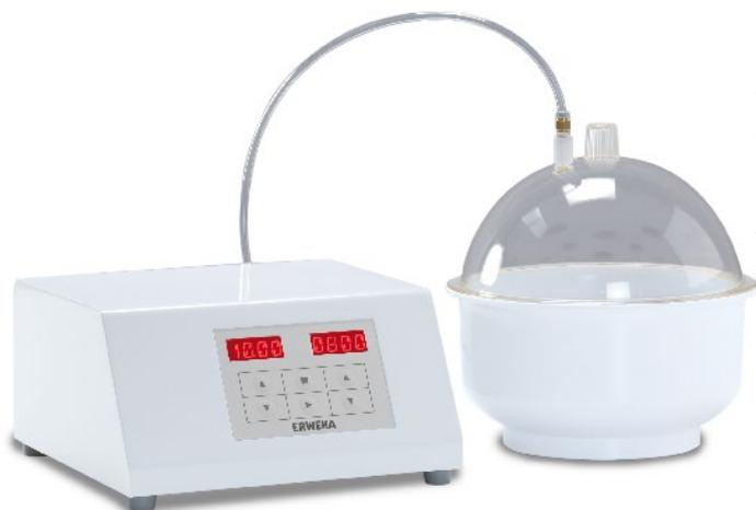
The ERWEKA VDT/S is a vacuum leak tester for blisters and other vacuum forms. With its compact size, the VDT is ideal for quality control during the packing and filling process. The ERWEKA VDT/S consists of two connected units - the main control unit with the integrated vacuum pump and the vacuum exsiccator (available in different sizes with 150, 200, 250 or 300 mm diameter).
